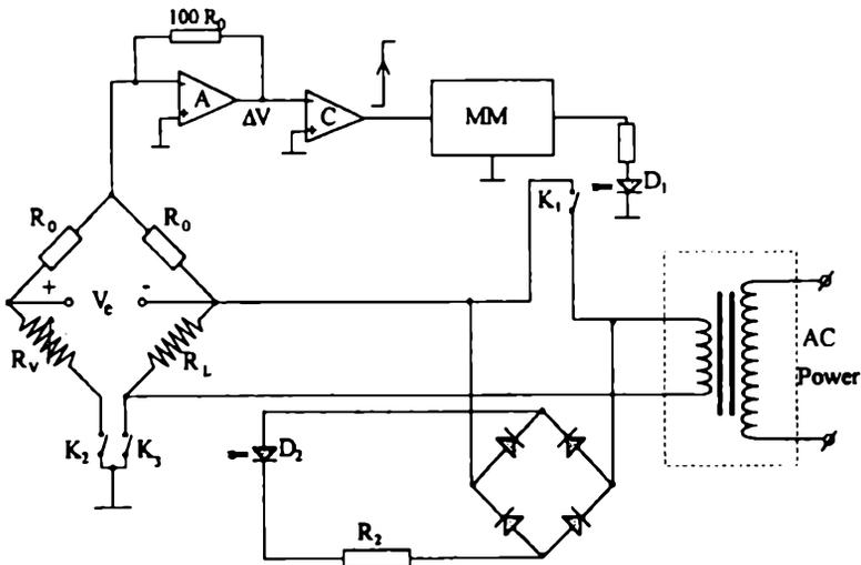
Fig. 2. Economic circuit with single switching device in AC power loop. Transformer is optional
