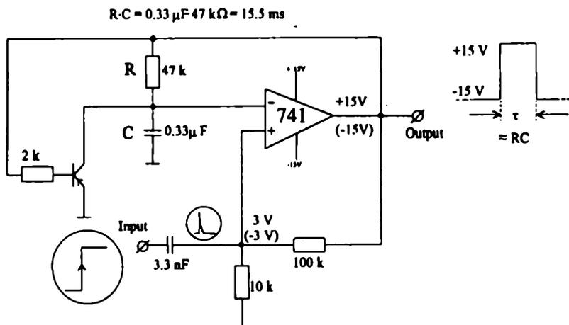
Fig. 5. Monostable multivibrator circuit based on operational amplifier 741 and p-n-p transistor (e.g. BC 393)
