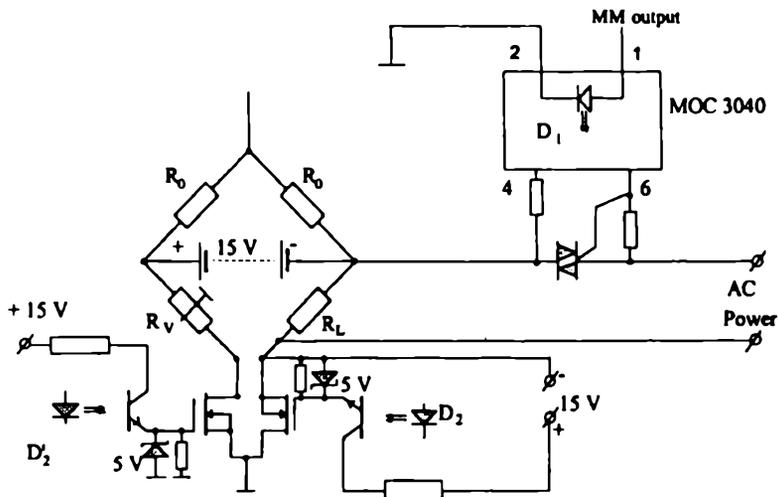
Fig. 3. Details of the switching devices  $K_1$ ,  $K_2$  and  $K_3$  from Fig. 2. Diodes  $D_2$  and  $D_2'$  are connected in series. Two MOSFET transistors and two optically coupled isolators CNY17 were used.
