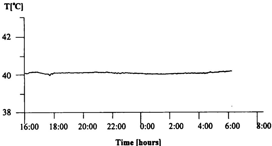
Fig. 6. Long-term test of temperature stabilisation
