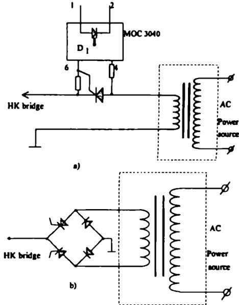
Fig. 4. Use of thyristors as switching devices: (a) half-wave rectifier, (b) full-wave rectifier. Transformer is optional
