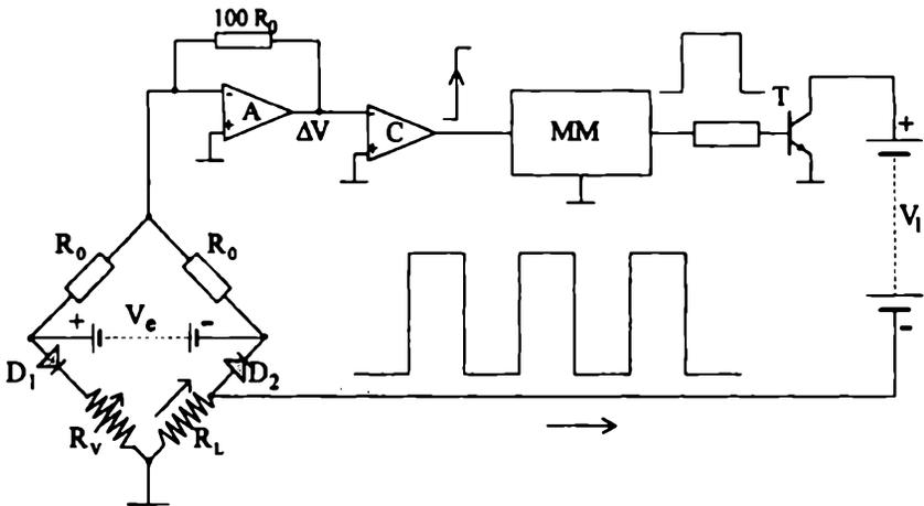
Fig. 1. Schematic diagram of new type monostable multivibrator for temperature control of load resistor ( $R_L$ ) making up one leg of Halas-Kaminski bridge.  $A$  — amplifier,  $C$  — comparator,  $MM$  — monostable multivibrator
