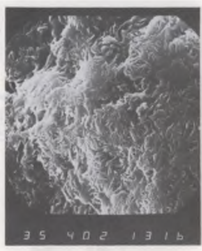
Phot. 5. Glauconite grain from 2.4-2.3 (g/cm 3 ) density fraction, magnification x 2500
