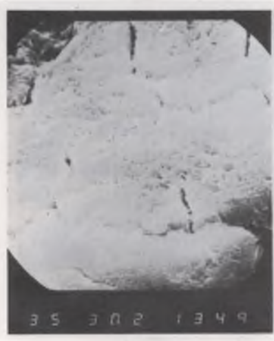
Phot. 4. Glauconite grain from 2.5-2.4 (g/cm 3 ) density fraction, magnification x 1900
