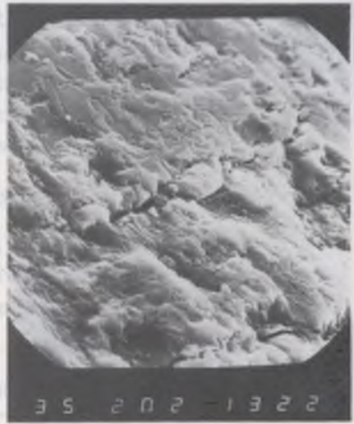
Phot. 2. Glauconite grain from 2.7-2.6 (g/cm 3 ) density fraction, magnification x 1200
