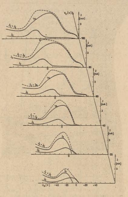
Fig. 3. The dependence current intensity of the collector  $I_c$ and cone electrode  $I_E$  versus the probe voltage  $U_s$ at the various potential  $V_E$ .
