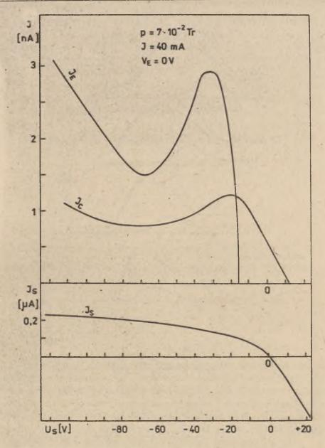
Fig. 2. Typical extraction probe characteristic I<sub>s</sub>=f(U<sub>s</sub>) and dependence current intensity of the collector I<sub>c</sub> and cone electrode I<sub>E</sub> versus the probe voltage U<sub>s</sub>.
