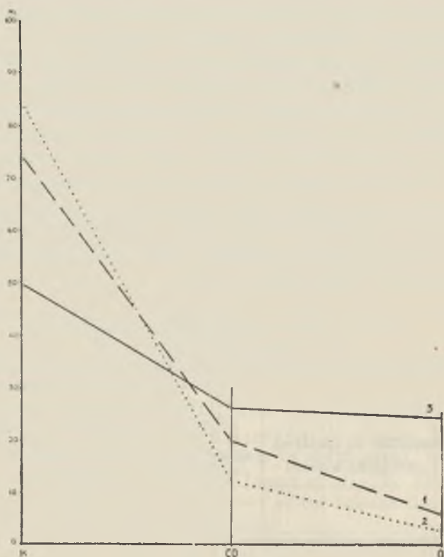
Graph 4. Morphology of quartz particles: 1 — Biecz waste, 2 — Biecz slate, 3 — loess of the Szczebrzeszyn, K — sharp-edged grains, CO — partly rounded grains, O — rounded grains.
