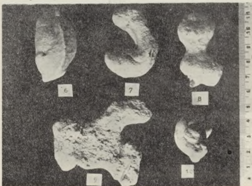
Fig. 2. Examples of the type of the shape of loess concretions; 6 — conchoidal, 7 — kidney-shaped, 8 — double, 9 — irregular, 10 — conglomeratic
