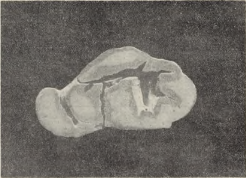
Fig. 4. The distribution of the clay minerals and of the calcite inside the concretion
