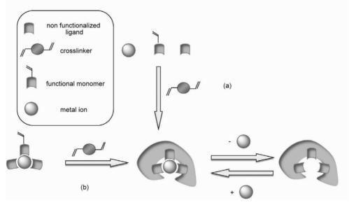
Fig. 6. Elaboration of IIPs trapping approach without (a) and with (b) prior formation of the complex between the template ion and ligand.
