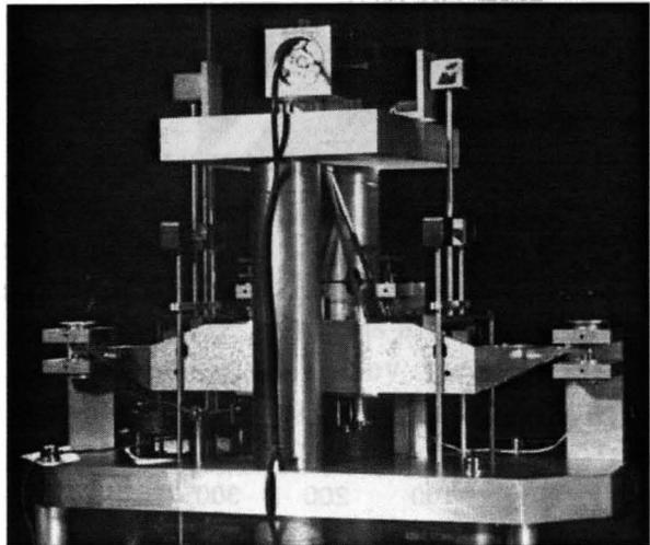
Fig. 9. Flexure-strip balance FB-2, © Bureau International des Poids et Mesures (BIPM), Sèvres, France.
