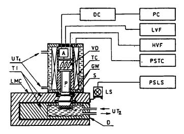
Fig. 2. Block diagram of measuring apparatus [8]: LMC — light-proof measurement chamber, TI — thermal insulator, D — drawer, S — sample, GW — glass windows, P — photomultiplier, VD — voltage divider, A — amplifier, DC — discriminator, PC pulse counter, LVF — low-voltage feeder, HVF — high-voltage feeder, PSTC — power supply of thermoelectric cooler TC, PSLS — power supply of light source LS, UT<sub>1</sub> and UT<sub>2</sub> — stub pipe for water addition from ultrathermostats
