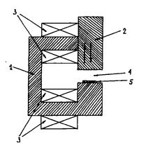
Fig. 1. Block diagram of electromagnet: 1 — magnetic core; 2 — mobile magnetic core; 3 — field coils; 4 — air gap; 5 — sample of seeds
